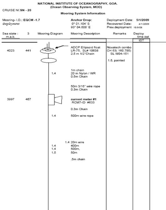
**Figure 1** OOS Current Meter Mooring sites CEIO (77°E, 83°E) and EEIO (93°E) in EEIO (left) and engineering structure of the mooring design. (Right).
