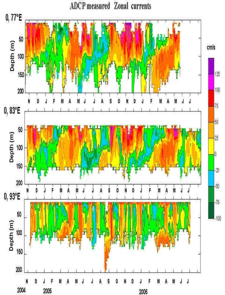
**Fig 2:** Zonal velocity structure of the WEIO, CEIO& EEIO location over Equatorial Indian Ocean (EIO).
