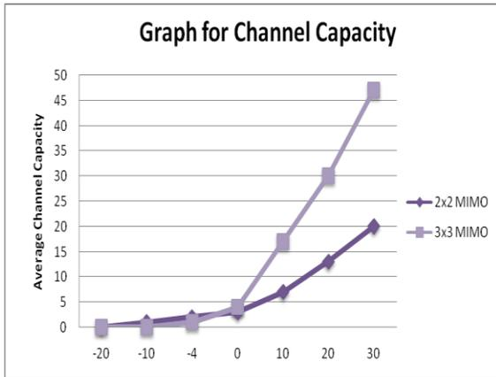
Fig. 2: Average channel capacity Vs. SNR for Rayleigh fading channel for 2X2 and 3X3 MIMO system
