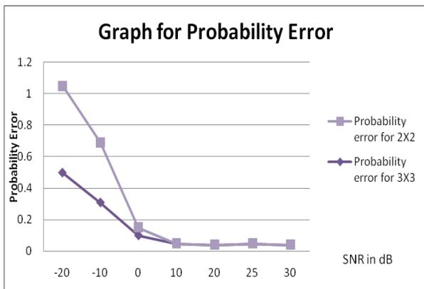
Fig. 3: Probability error VS. SNR for 2X2 and 3X3 antenna for
