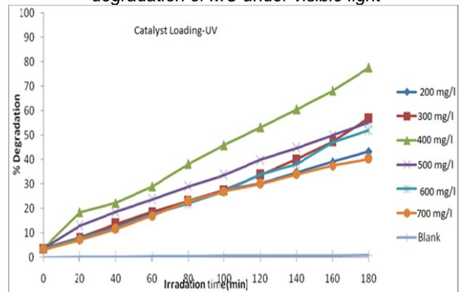
Figure 10. Effect of catalyst loading for photocatalytic degradation of MO under UV irradiation.
