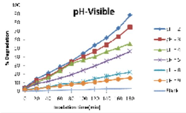
Figure 7. pH effect on the photodegradation of MO under visible irradiation
