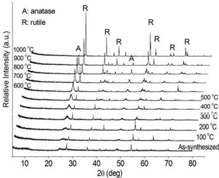
**Fig. 2** XRD patterns of the prepared sample calcined at various temperatures
