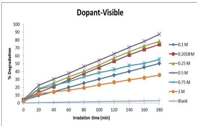
Figure 5. Effect of Ag concentration under visible light.
