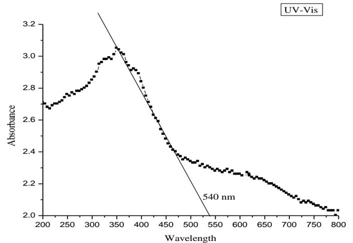
**Figure.4** UV/Vis absorbance edge of ANT
