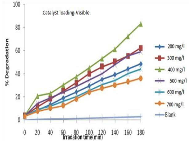
Figure 9. Effect of catalyst loading for photocatalytic degradation of MO under visible light
