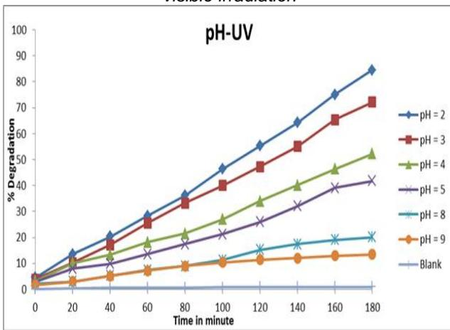
Figure 8. pH effects on the photodegradation of MO under UV irradiation.
