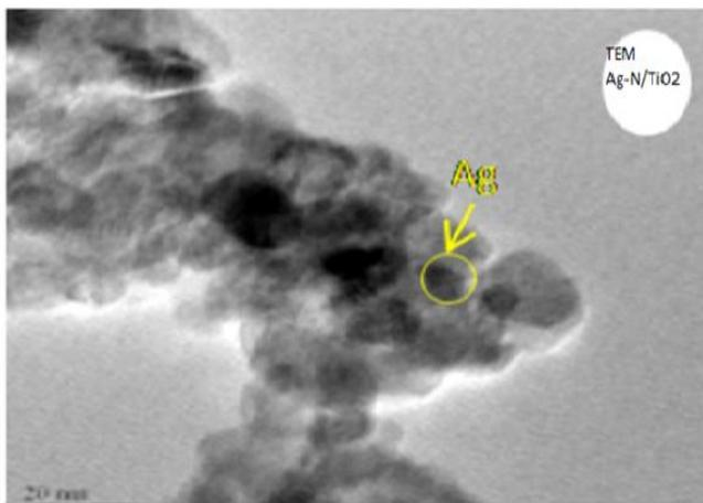
**Fig. 3** TEM image of Ag-N co-doped TiO<sub>2</sub>
