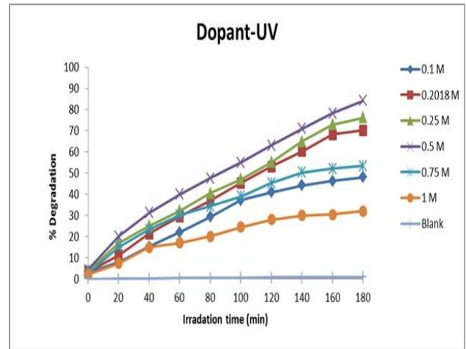
Figure 6. Effect of Ag concentration under UV irradiation.
