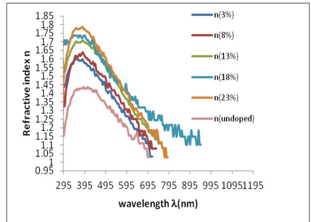
**Fig. 4:** Variation of refractive index with percentage doping for  $MgCo_2O_4$  nanofilm.
