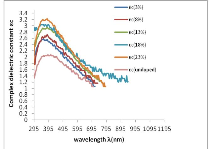
**Fig. 7:** Variation of Complex dielectric constant with percentage doping for MgCo<sub>2</sub>O<sub>4</sub> nanofilm.
