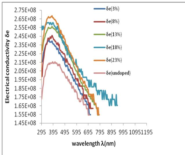
**Fig. 6:** Variation of electrical conductivity with percentage doping for MgCo<sub>2</sub>O<sub>4</sub> nanofilm.
