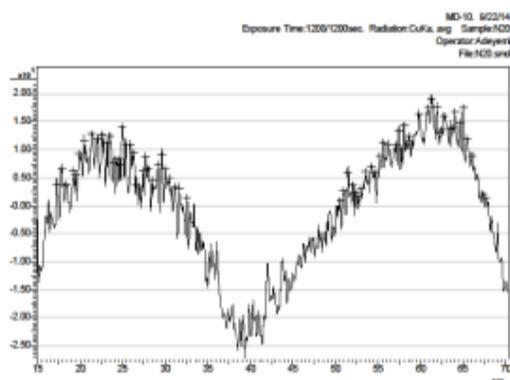
Fig. 10: XRD Pattern of MgCo<sub>2</sub>O<sub>4</sub> nanofilm
