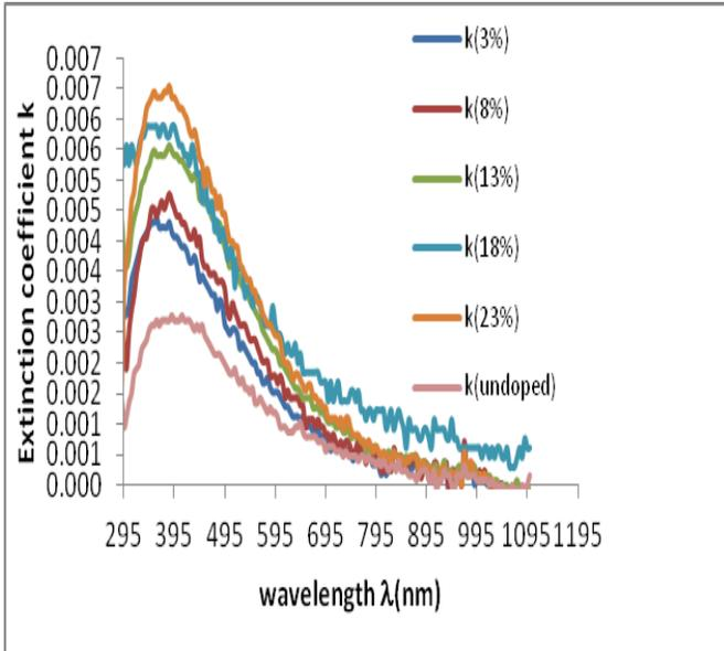
**Fig. 5:** Variation of extinction coefficient with percentage doping for MgCo<sub>2</sub>O<sub>4</sub> nanofilm.
