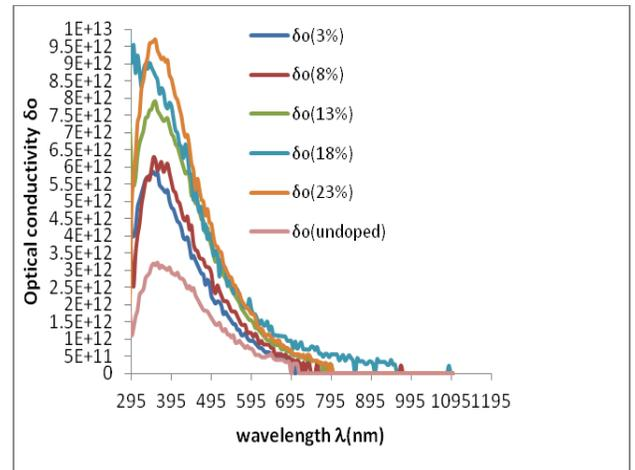
**Fig. 8:** Variation of Optical conductivity with percentage doping for MgCo<sub>2</sub>O<sub>4</sub> nanofilm
