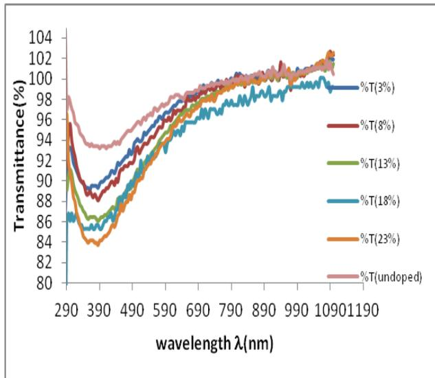
**Fig. 2:** Variation of transmittance with percentage doping for  $MgCo_2O_4$  nanofilm.
