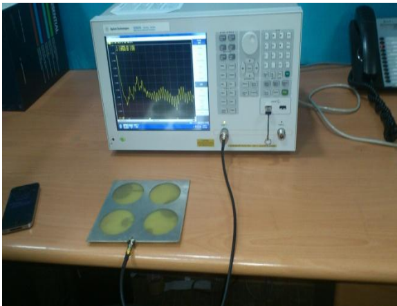
Fig.8 Testing of multibeam antenna array using vector analyzer
