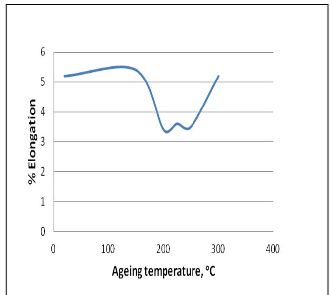
**Fig.3.** Variation of the ductility (% elongation) with the ageing temperature of the alloy
