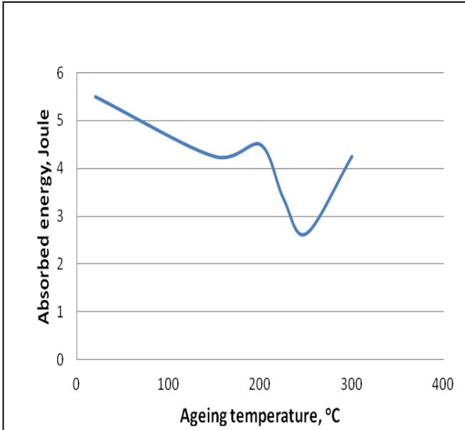
**Fig. 4.** Variation of the impact energy with the ageing temperature of the alloy
