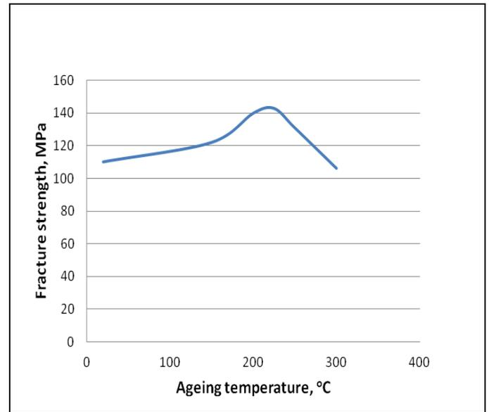
**Fig.2.** Variation of the fracture strength with the ageing temperature of the alloy
