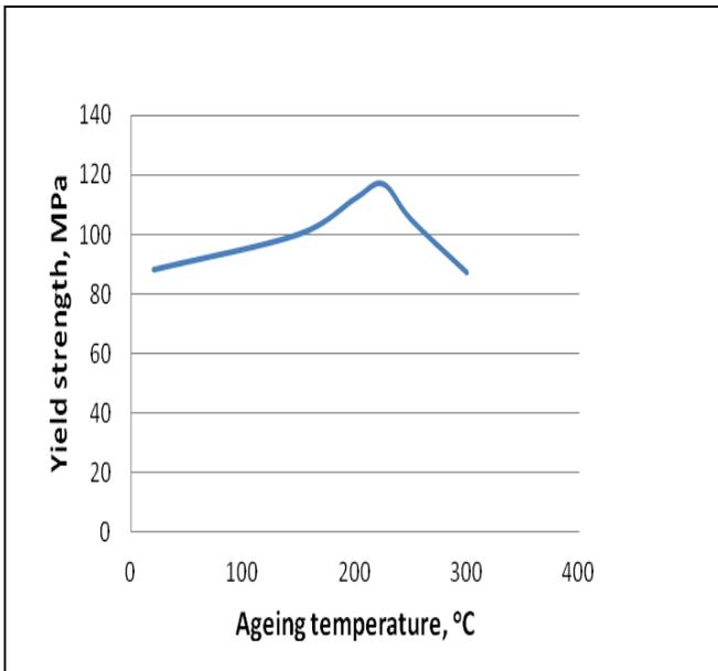
**Fig.1.** Variation of the yield strength with the ageing temperature of the alloy.
