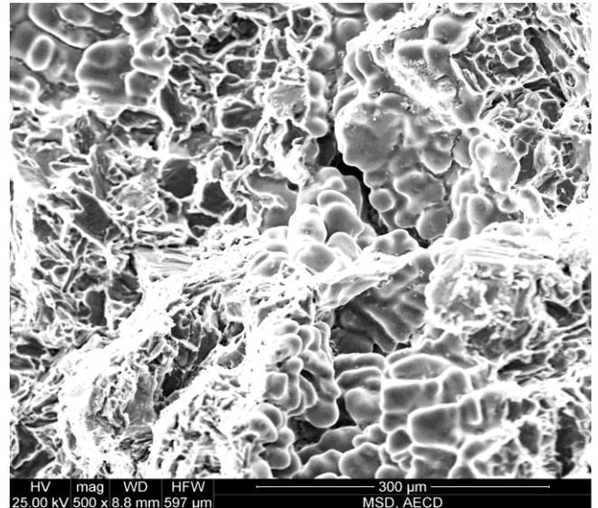
**Fig. 5.** SEM tensile fracture surface of Al-6Si-0.5Mg alloy at solution treated condition.
