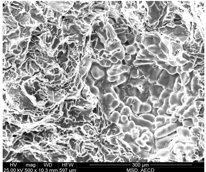
**Fig. 6.** SEM tensile fracture surface of Al-6Si-0.5Mg alloy at peak aged condition.
