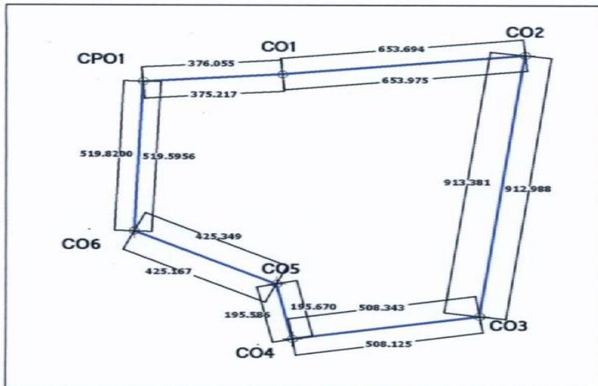
Fig.3. 1: Total Station and GPS common points traverse
