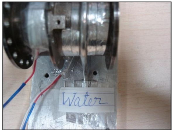
Figure 10 Single Curve two Heat Pipe at \theta = 90^\circ on Cavity
