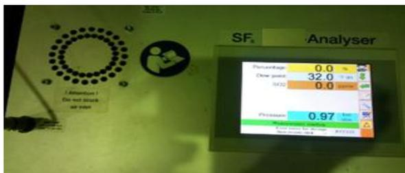
Fig. 9 SF6 Gas analyzer tester (SF6 MULTI-Analyser)
