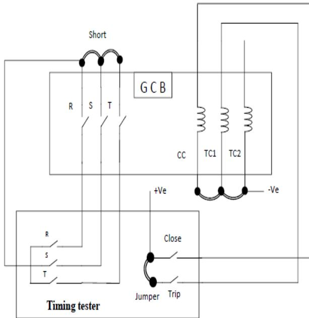
Fig3. Connection test timing with the circuit breaker
