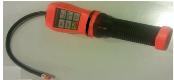
Fig.10 Gas leakage tester instrument
