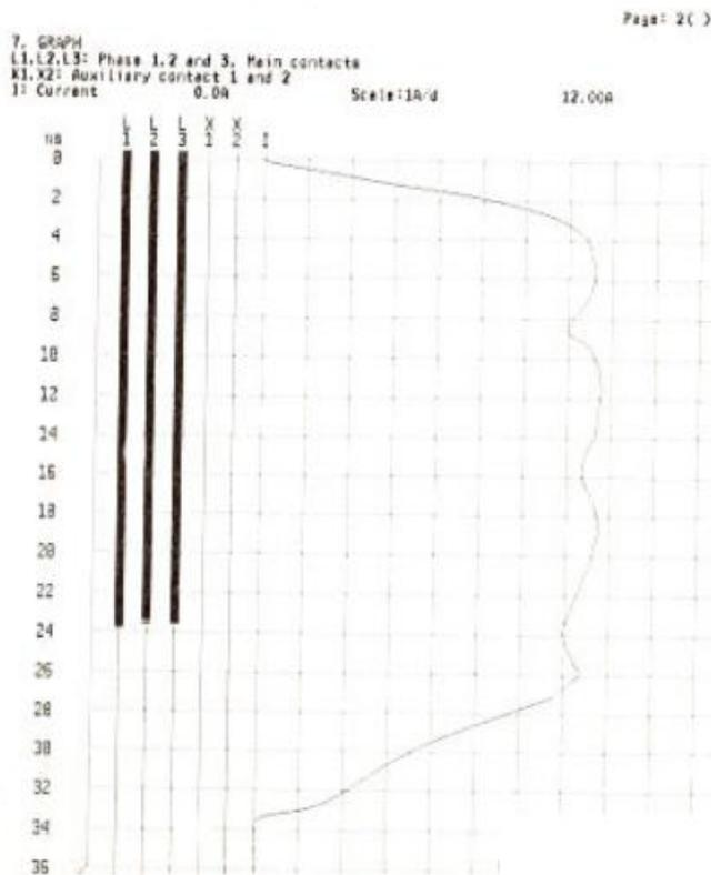
Fig.5 open circuit breaker test (by trip coil 1)
