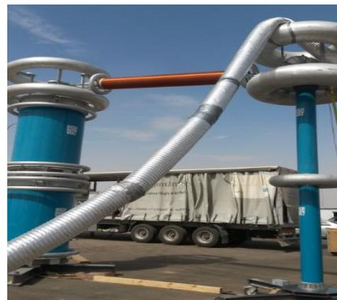
Fig. 11 High voltage tester
