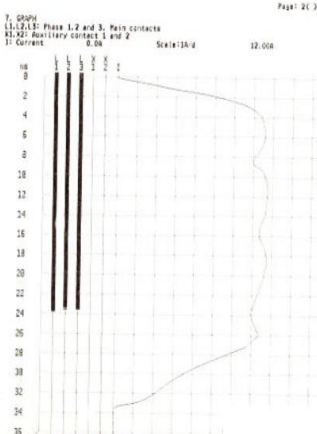
Fig.6 open circuit breaker test (by trip coil 2)
