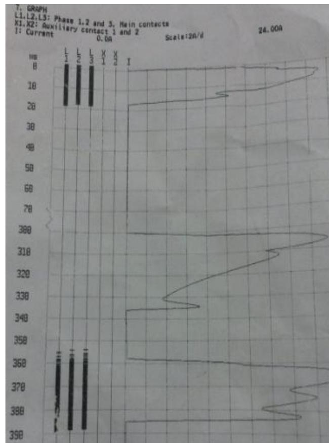
Fig.7 open close open printed test sheet
