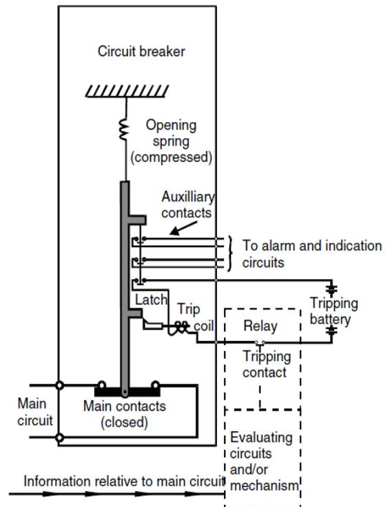
Fig. 1 Design for the high voltage circuit breaker
