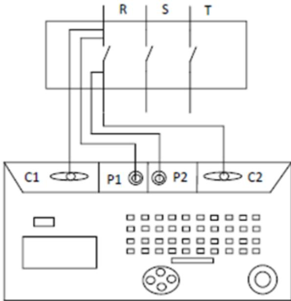
Fig.8 the connection for the contact resistance test
