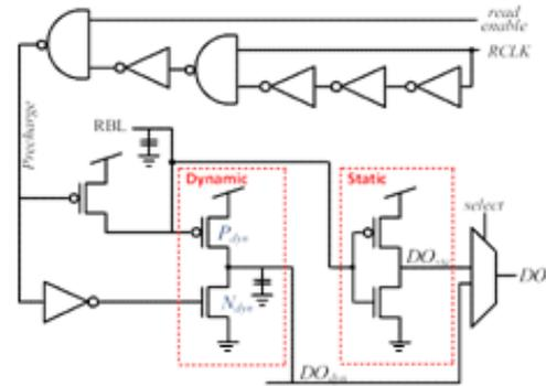
**Fig.4.** Dynamic readout architecture (c)
