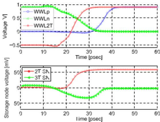
**Fig.3.** Effects of CI and CF mechanisms. (a) Conventional 2T bitcell. (b) Proposed 3T bitcell. (c) Waveform comparison of the two bitcells during write deassertion
