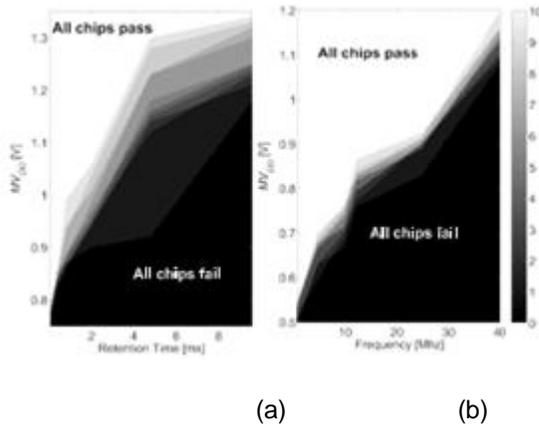
**Fig.6. Minimum memory supply voltage Shmooplots for 10m measured chips. (a) Minimum MVDD versus DRT. (b) Minimum MVDD versus frequency.**
