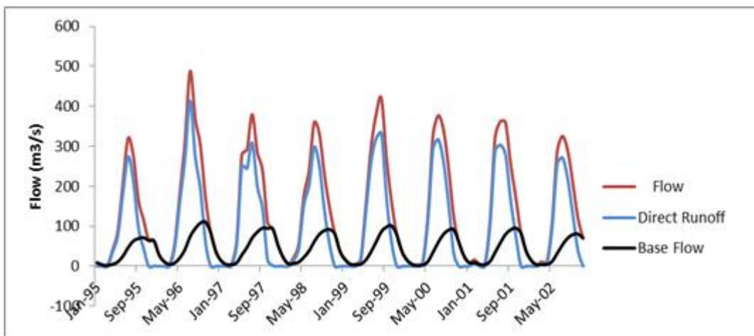
**Fig.4.4** Direct runoff and Base flow hydrograph of Gilgel Abay Watershed
