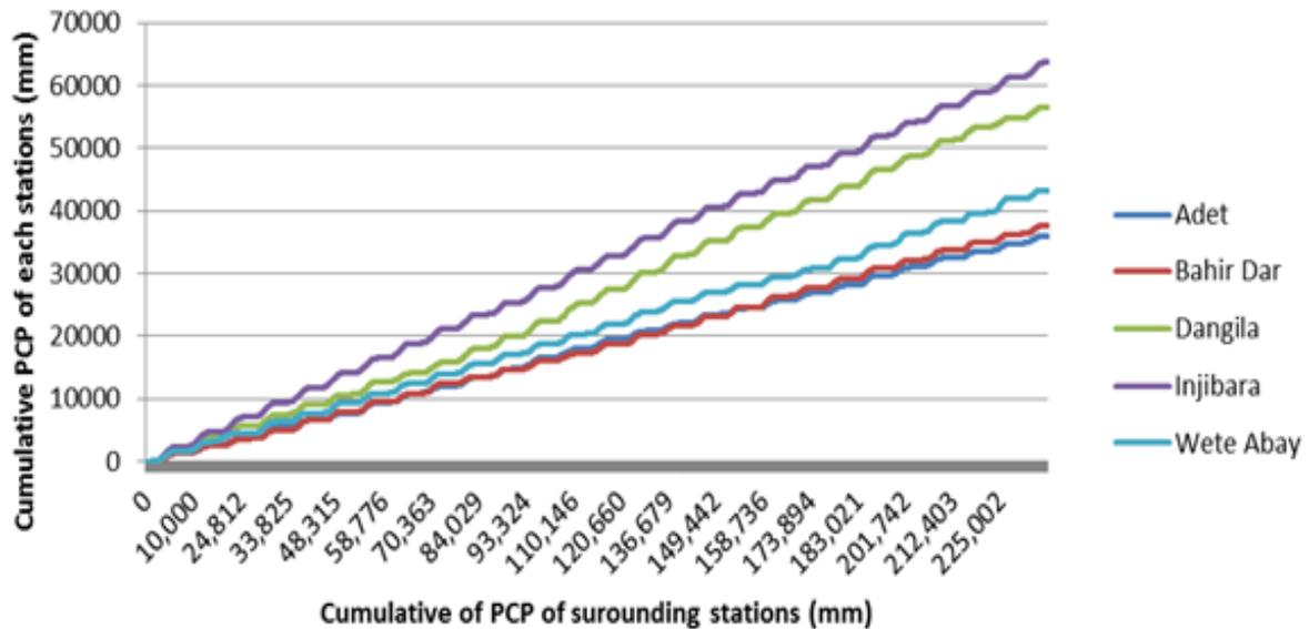
Figure 3. 2 Double mass curve showing homogeneity of precipitation gauges data
