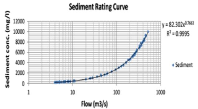
Fig. 3. 1Discharge vs. Sediment Rating curve developed for Gilgel Abay Watershed
