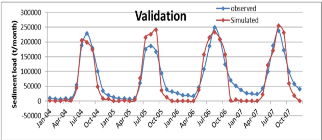
Fig. 4.7 Comparison of observed vs. simulated sediment yield results for the validation period (2003 - 2007) using 1986 land use
