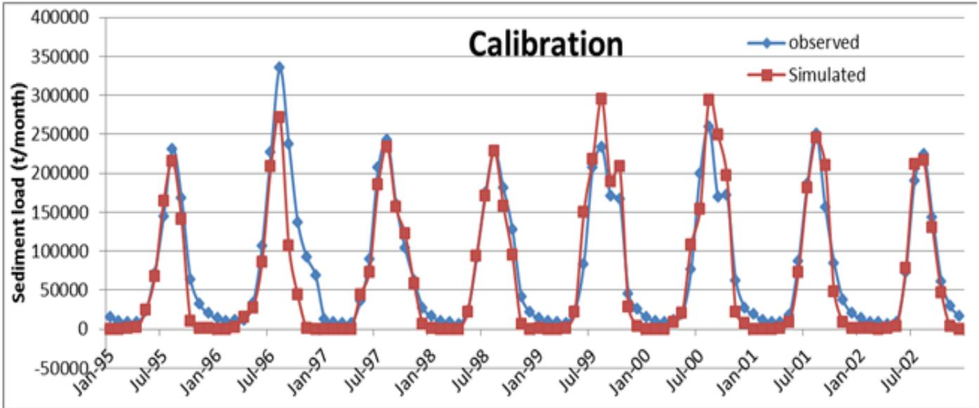
Fig.4.6 comparison of measured vs. simulated sediment yield results of the calibration period (1995 - 2002) using 1986
