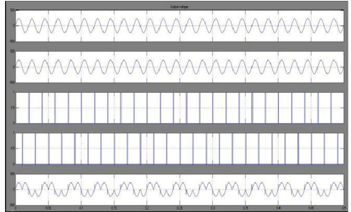
**Figure-2** Voltage Waveform shows the input frequency is 2 times the output frequency for thyristor
