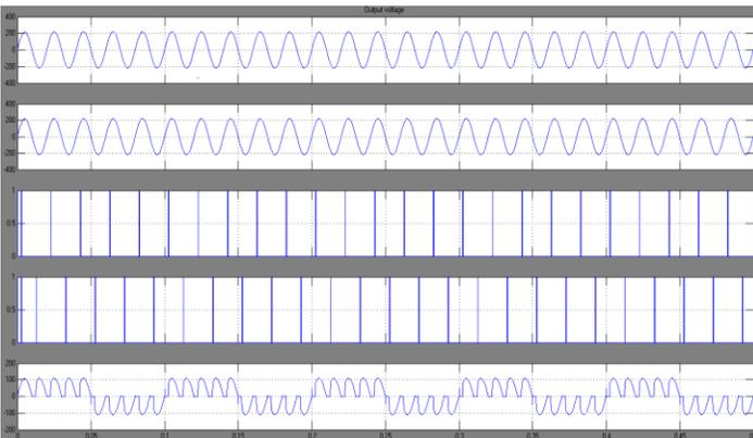
**Figure-4** Cycloconverter output for 30° firing angle
