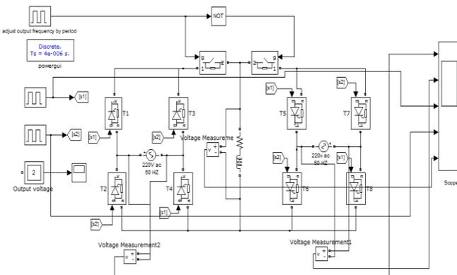
**Figure-1** Single phase cycloconverter Thyristor combination
