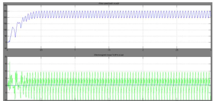
**Figure-10** Wave shapes of rotor speed and torque at 12.5Hz
