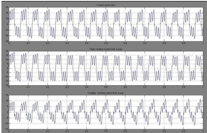
**Figure-6** Wave shapes of output currents across the motor (output frequency is one third of input frequency)
