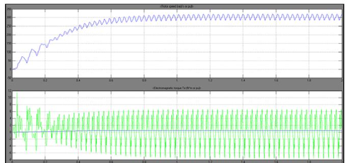
**Figure-9** Wave shapes of rotor speed and torque at 16.67Hz
