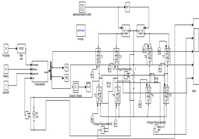
**Figure-3** Cycloconverter with firing angle system
