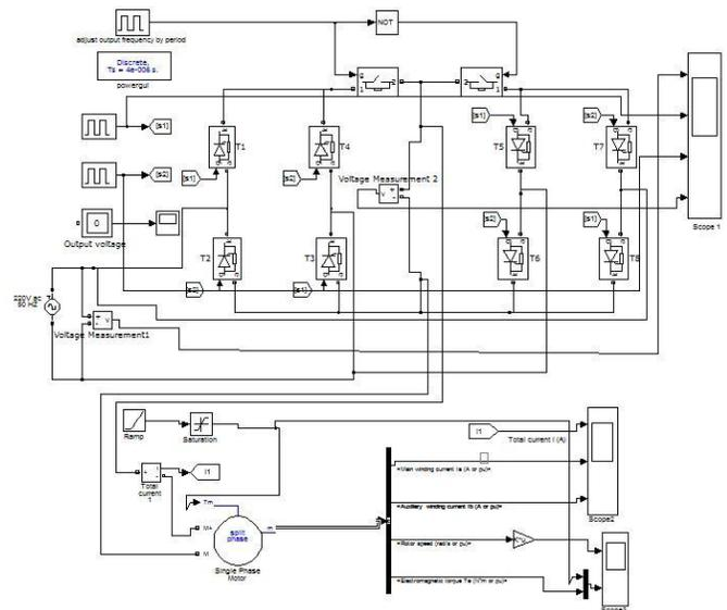
**Figure-5** Cycloconverter with Split phase Induction motor
