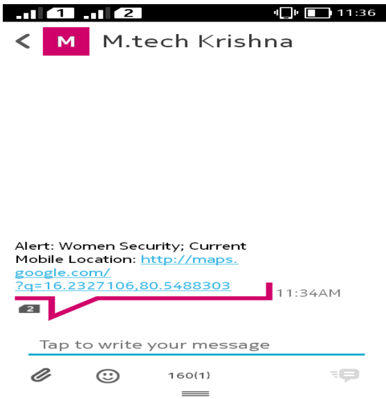
Fig.5. Message received by another contact device immediately after starting the application.
