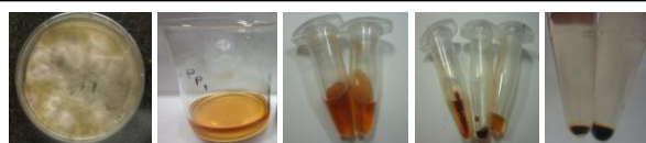
Fig. 1 Silver nanoparticle bio-synthesis using extracellular fungal secretes (a) Penicillium pinophilum culture in PDA media, (b) Fungal secretes after synthesis of AgNPs (c) AgNP suspension, (d) AgNP palates after centrifugation at 12000rpm (d) Ag nanoparticles.
