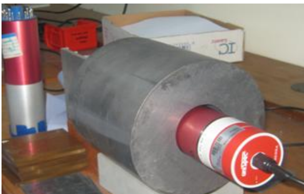
Fig1: The NaI (TI) detector with cylindrical lead shield surrounding it
