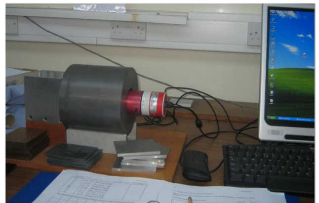
Fig3 The shield material, the NaI(Tl) detector and the connections to the monitor
