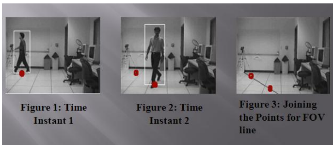
Fig(8) -Plotting the Edge of FOV lines when cameras are not in Parallel
