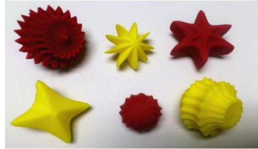
Fig. 6. Supershapes printed using FDM machine
