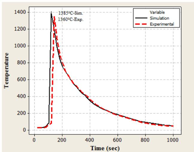
**Figure 12.** Comparison of simulation and experimental thermal profiles.
