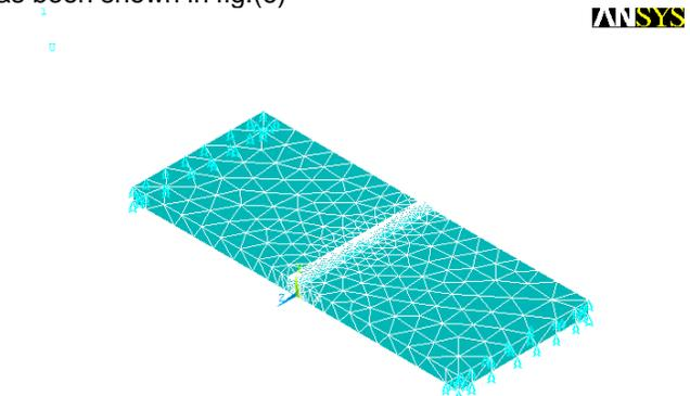
**Figure 6.** Structural boundary conditions
