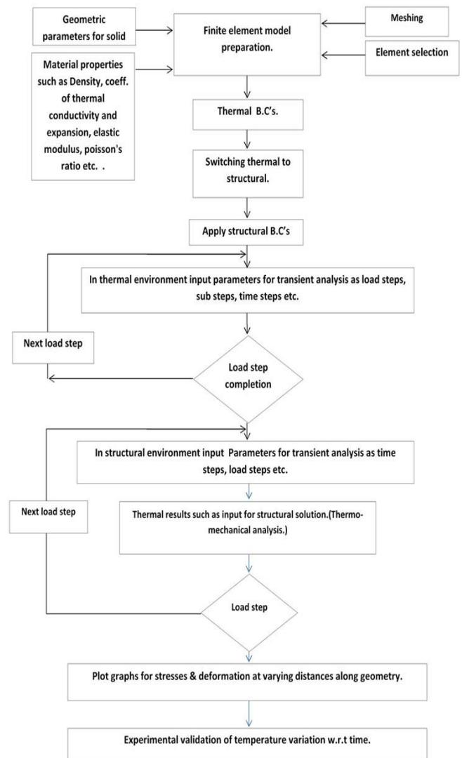
**Figure 2.** Flowchart of simulation procedure
