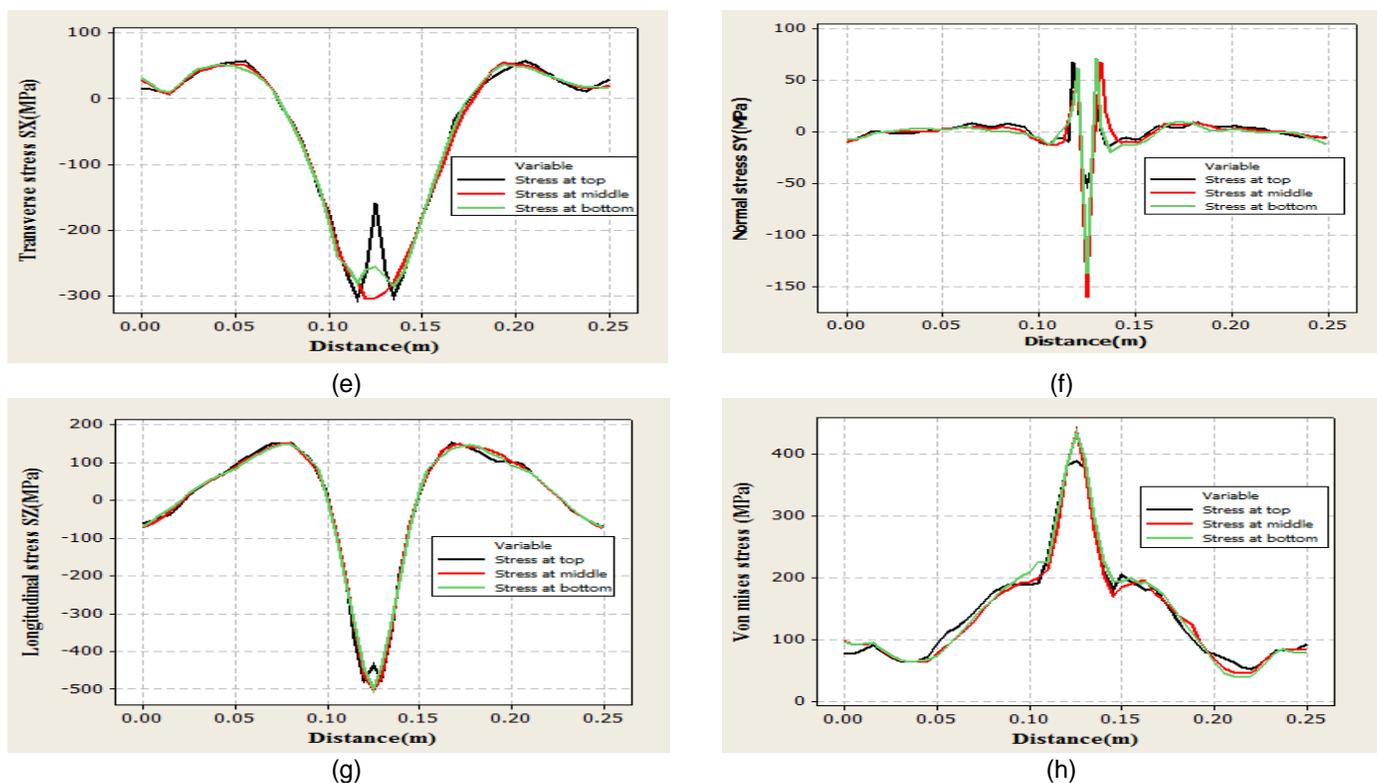
**Figure 11.** Stress distribution across the weld bead at the middle section ( $z = 50\text{mm}$ ) along thickness: (a) transverse stress SX, (b) normal stress SY, (c) longitudinal stress SZ, and (d) Von Mises stress SEQV.
