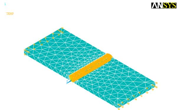
**Figure 5.** Thermal boundary conditions
