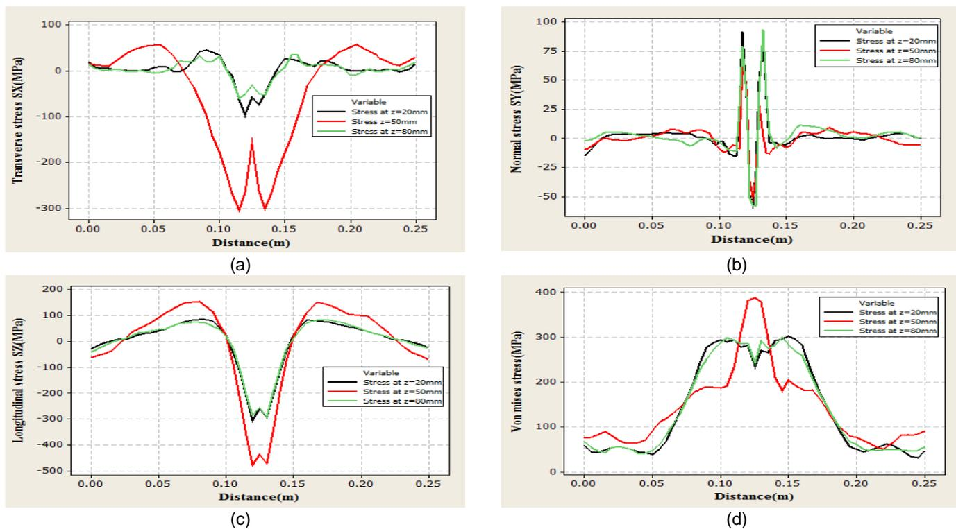
**Figure 10.** Stress distribution along weld bead at three different paths at the top surface of weld bead obtained by GMA welding: (a) transverse stress SX, (b) normal stress SY, (c) longitudinal stress SZ, and (d) Von Mises stress SEQV.
