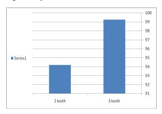
[2] The following chart gives a comparison between three and two teeth concave for material capacity
