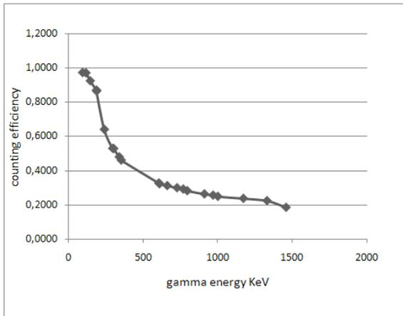
Fig. 1-Efficiency of well-shape 2x2 NaI(Tl) detector
