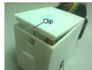
Fig. 16. Insertion of top cover to enclose the segment block.
