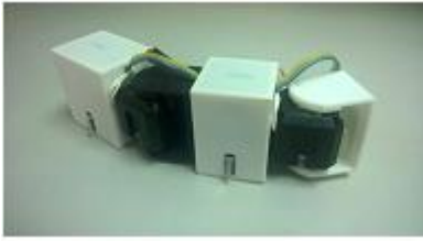
Fig. 17. Overview of constructed snake-like modular robot assembled with different body parts.
