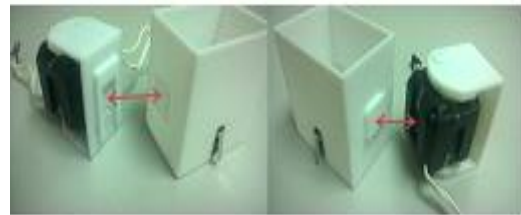
Fig. 14. Connection parts between segment block and actuator joint.
