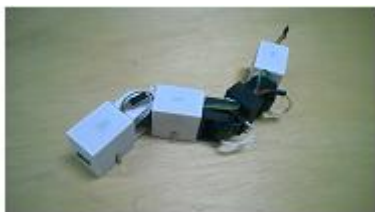
Fig. 18. Fully constructed 4-segment lateral undulation snake-like modular robot.
