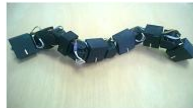
Fig. 22. Fully constructed 7-segment lateral rolling snake-like modular robot.
