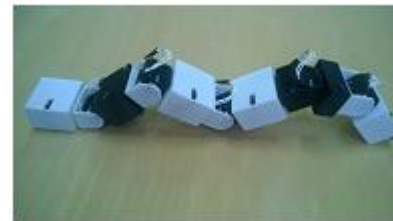
Fig. 20. Fully constructed 6-segment vertical undulation snake-like modular robot.
