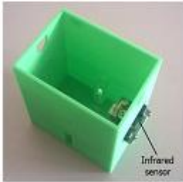
Fig. 10. First segment block fabricated.
