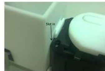
Fig. 15. Insertion of wedge connector into bracket slot.
