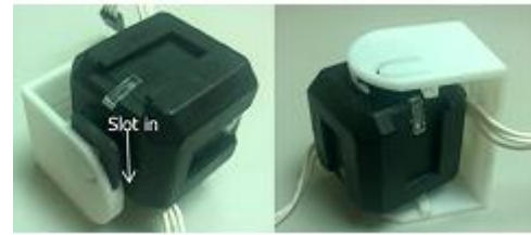
Fig. 13. Insertion of servo motor into joint connector.
