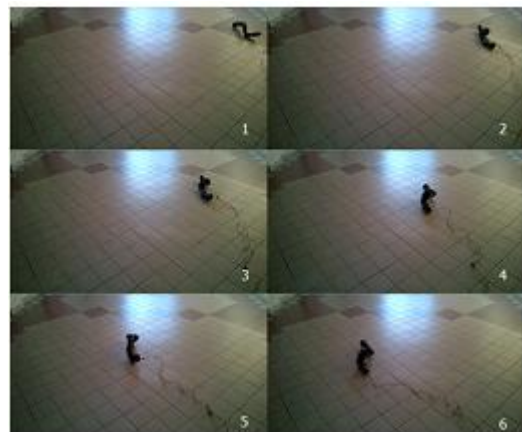
Fig. 23. Lateral rolling moving behaviour performed by 7-segment snake-like modular robot.
