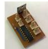
Fig. 8. Fabricated shift register circuit board.
