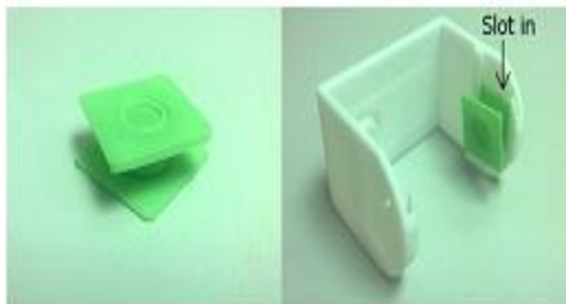
Fig. 12. Fabricated rotation connector.
