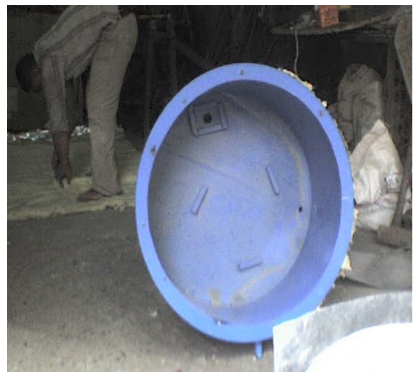
Fig. 3: The jacket of the vessel with the opening through which the valve is assembled shown.
