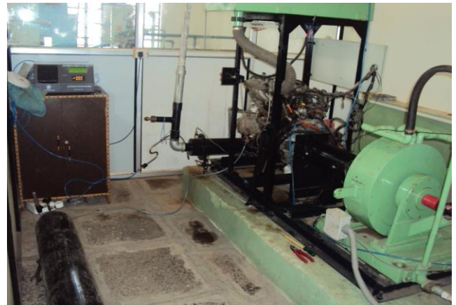
Fig 3: Photograph of computer controlled 4 stroke SI engine test rig with Experimental set-up.
