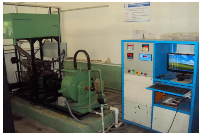
Fig 4: Photograph of computer controlled 4 stroke SI engine test rig with control panel.
