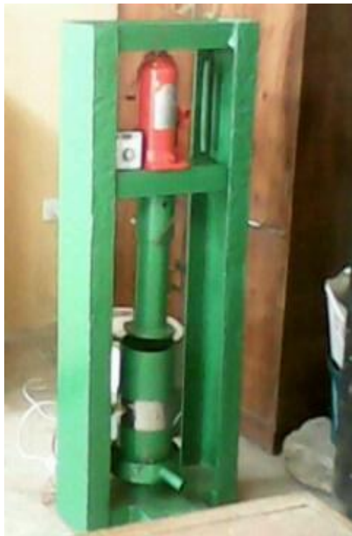
Fig (1): Pictorial View of the Spring-Controlled Hydraulic Press Used for the Study.
