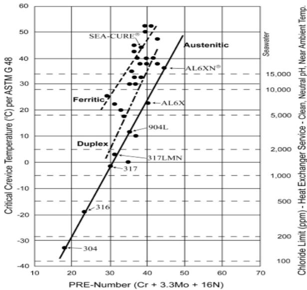
**Figure3: Critical Crevice Temperature and Maximum Chloride Levels versus PREn of Various Stainless Steels**
