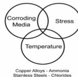
**Figure2:** production of corrosion in the heat exchanger surface. [2]
