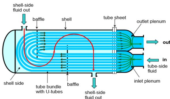
**Figure1-** Heat Exchanger [1]
