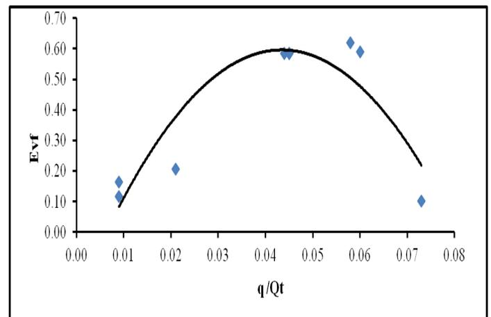
**Figure 5:** Behavior of  $E_{vf}$  versus  $q/Q_t$  when  $H = (1.5 - 6) m$ ,  $f = (30 - 120) \text{ beats/min}$ ,  $V_s = (2.45 - 19.6) \text{ litres}$ ,  $h_3 = (20 - 120) m$  and  $L = 18.5 m$
