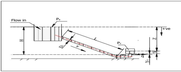
**Fig. 1:** A setup model for a conventional hydram pumping system.
