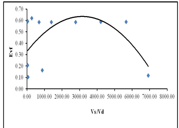
**Figure 4:** Behavior of  $E_{vf}$  versus  $V_s/V_d$  when  $H = (1.5 - 6) m$ ,  $f = (30 - 120) \text{ beats/min}$ ,  $V_s = (2.45 - 19.6) \text{ litres}$ ,  $h_3 = (20 - 120) m$  and  $L = 18.5 m$
