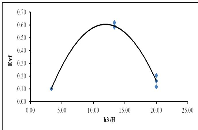
**Figure 2:** Behavior of  $E_{vf}$  versus  $h_3/H$  when  $H = (1.5 - 6) m$ ,  $f = (30 - 120) \text{ beats/min}$ ,  $V_s = (2.45 - 19.6) \text{ litres}$ ,  $h_3 = (20 - 120) m$  and  $L = 18.5 m$
