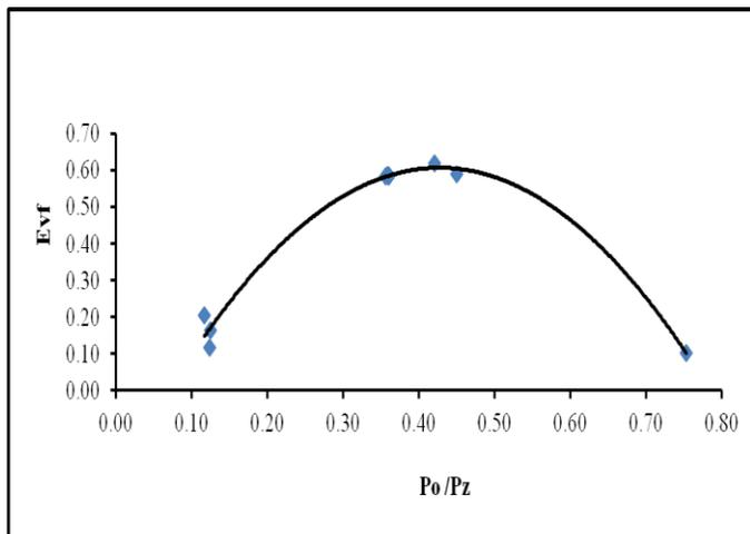
**Figure 3:** Behavior of  $E_{vf}$  versus  $P_o/P_z$  when  $H = (1.5 - 6) m$ ,  $f = (30 - 120) \text{ beats/min}$ ,  $V_s = (2.45 - 19.6) \text{ litres}$ ,  $h_3 = (20 - 120) m$  and  $L = 18.5 m$
