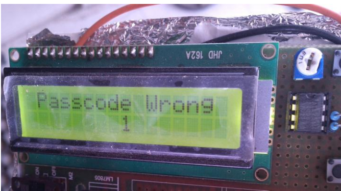
Passcode wrong indicating once in LCD display
