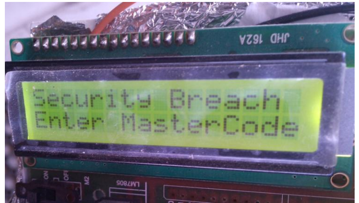
Showing the Security breach enter password in LCD display
