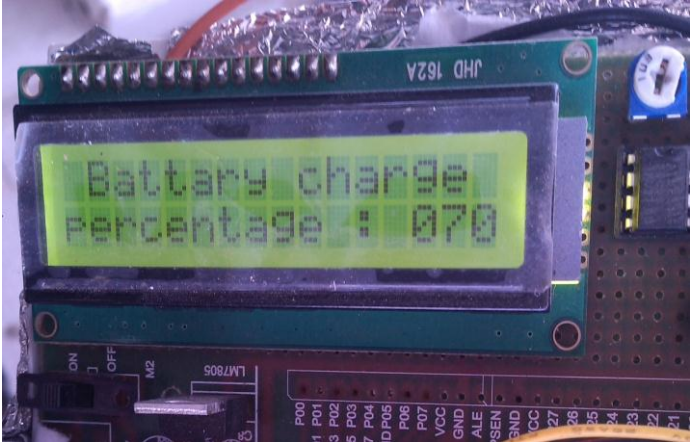
Battery Level varying from 080% to 70%
