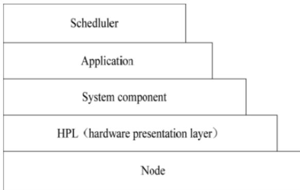
Figure 5 : The framework of TinyOS
