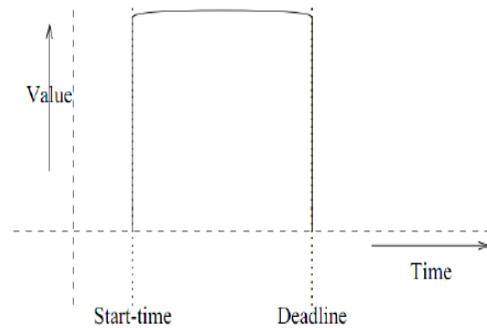
**Figure 2:** common characteristic of real-time systems
