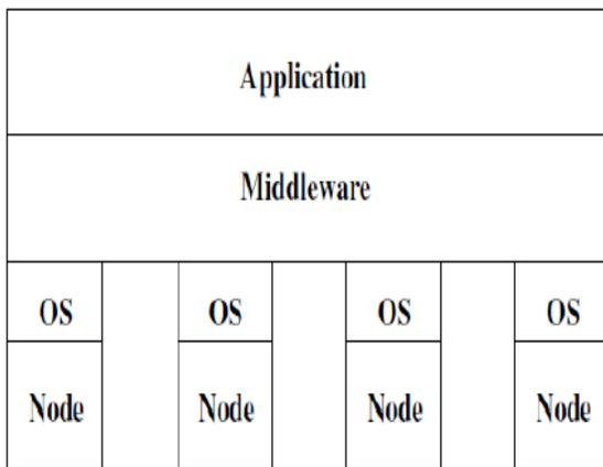
**Figure 1:** operating system stands in the software layers of the WSN
