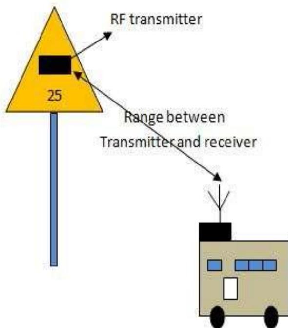
**Figure 1:** Traffic Signal posts equipped with RF Transmitter (left) Automobile equipped with the RF receiver (right)
