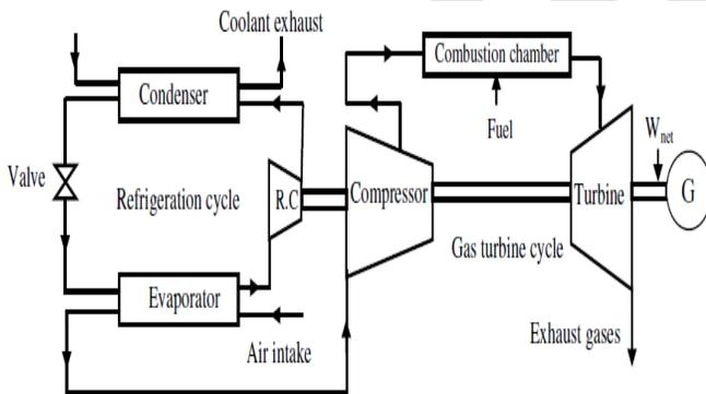
This system consumes more power to drive compressor and pumps. The initial cost of the machine is high and slightly maintenance cost also high.
