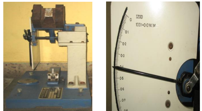
Fig-5: Model K-1.4 impact machine
