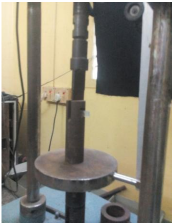
Fig-7: Double shear test in UTM
