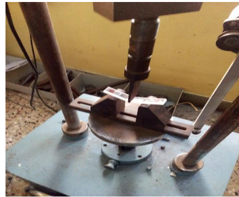
Fig-4: Flexural test in UTM
