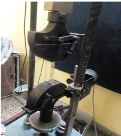
Fig-3: Tensile test in UTM
