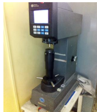
Fig-6: Rockwell L-scale machine
