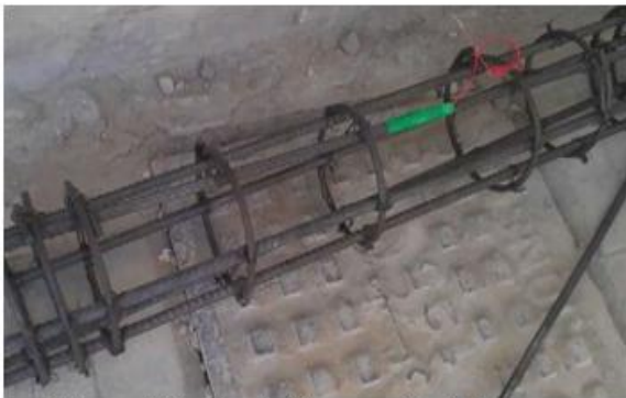
Figure ( 2 ) : Strain Gauge on Steel Cage
