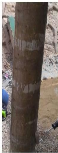
Figure ( 8 ) : Specimen with GFRP Strips Figure ( 9 ) : Specimen with GFRP Jacket
