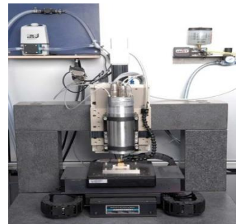
Fig. No. 2 Micro milling set up
