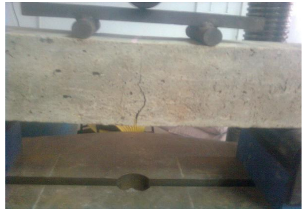
FIGURE 7 Crack on specimen after testing of specimen
