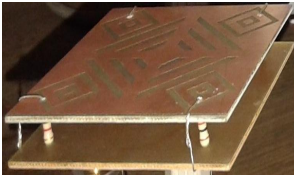
Fig. 7 Fabricated microstrip antenna with FSS and slotted patch
